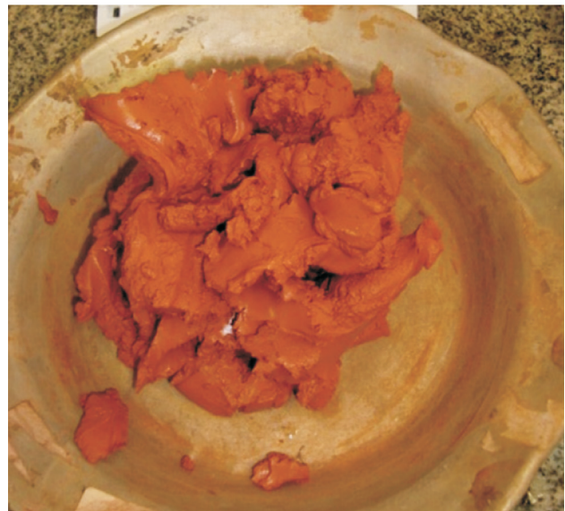
Figure 13 - Consistency states of the tailings tested (before and after the EKC test).
